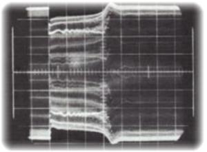
The oscillograph shows the ability of the LIMA®MAC to start Code G three phase motors. With 1 hp/kW across the line, there is less than a 35% voltage dip and fast recovery to rated voltage. The proportional volts/hertz characteristic with variations in shaft speed is ideal for induction motors.
