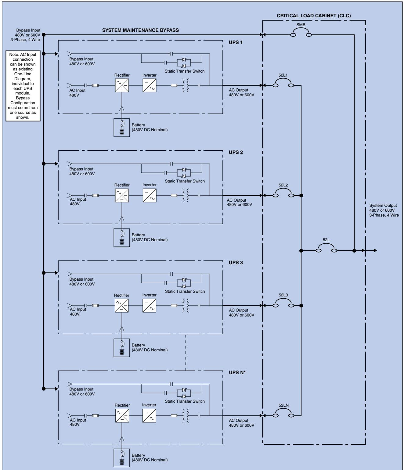
\*Up to 8 UPS modules (of same capacity) can be paralleled together in an MMS.
